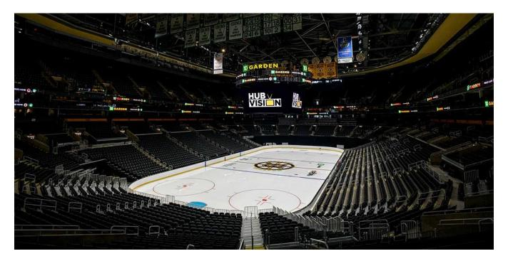
Above the 4K video boards, two new ring displays were installed on their own hoist system to allow them to be raised and lowered for the needs of the many events held at the venue. These displays each measure 3.5 feet high 179 feet in circumference and feature 3.9-millimeter pixel spacing.
