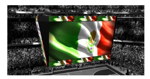
This artist's conceptual shows the design and configuration of the suspended centerhung video scoreboard. Measuring approximately 13.9 meters high by 23.8 m wide (46' x 78') and weighing more than 68,000 kilograms (150,000 lbs), it will be among the very largest and most capable of any in the world.
