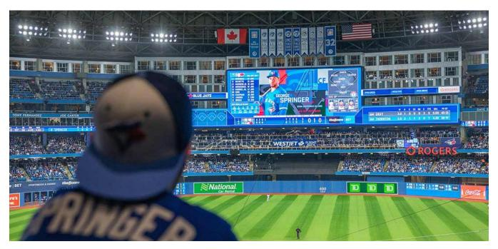
Flanking the main display are four additional LED displays and content can be coordinated across all five displays for one main center field viewing experience. Two displays mounted even with the bottom of the main display measure 15.5 feet high by 75.5 feet wide and two ribbon-style displays appear to extend out from the middle of the main display measure nearly 5 feet high by 75.5 feet wide. All center field displays feature 10-millimeter pixel spacing.
